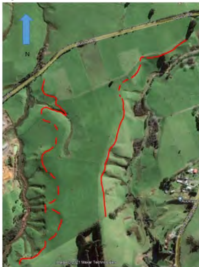
Figure 3: Image from Google Earth (date July 2015). Solid red lines illustrate inferred extent of weakly cemented resistant sand layer as exposed at the surface. Dashed lines signify where the sand layer is possibly less cemented and subject to headward gully erosion. Evident is the water springs which appear to align with the cemented sand horizon.
