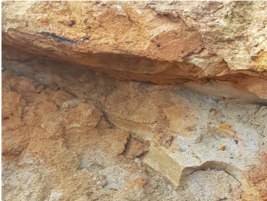
Photo 2: Weakly cemented sand material overlying clayey silt exposed in the quarry. The clayey silt has been subject to preferential erosion compared to the sand above most likely due to frittering on stress relief joints. This fine-grained material, including some organics, filled a small depression under the weakly cemented sand. This preferential erosion of layers is also seen near the subject site.
